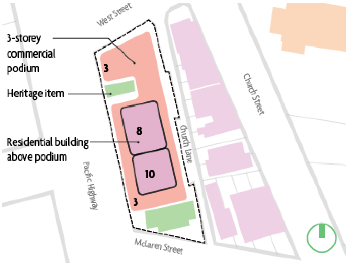
Figure 25 CPPS Building Envelope Plan – Subject Site
